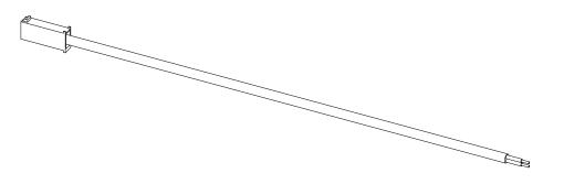
**Purpose:** 2-conductor cable that makes the electrical connection between the LED driver and the LINE sheets with a mating plug connector (required).
